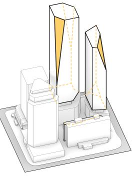
The tower forms respond at the scale of the city to solar control planes, enabling sunlight penetration deep into the site. The carved planes also enable the project to acknowledge its wider physical and cultural context - with the three primary chamfers conceptually making reference to the waters of the Kaipara, Manukau, and the Waitemata. The reflected sunlight in the glass planes acknowledges the energy created by te ara o te rā (the stations of the sun), and figuratively animates the
